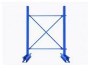
Step 3: Install connecting rod
