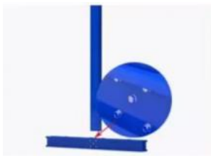
Step 1: Column inserted into the base and screw fixation
